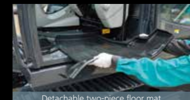
Detachable two-piece floor mat with handles for easy removal. A floor drain is located under floor mat.
