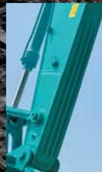
Specially designed long, solid rock guards installed to prevent damage to arm.
