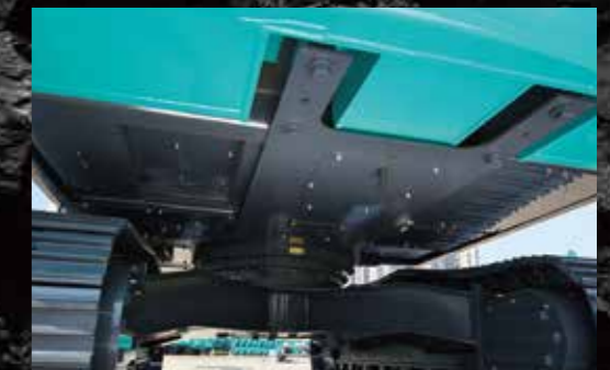
Thick covers with increased durability compared to standard models.
